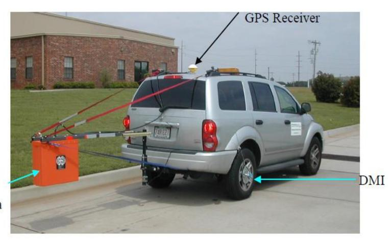
1 GHz Horn Antenna
